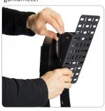
Before measurement, simply slide, align and lock the light source to the center
