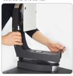
The base center lock makes it easy to align the light source to the center of rotation
