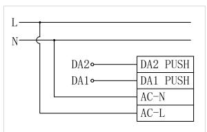
Wiring Diagram of DALI Dimming
