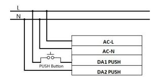
⚠ Remark: Before using PUSH dimming function, please connect AC-L/AC-N to electricity FIRST, then connect the PUSH terminal to electricity. Otherwise the PUSH terminal will be burned.
