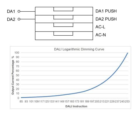
The DALI dimming function and the push dimming function cannot be used at the same time, otherwise the DALI dimmer will be damaged.
