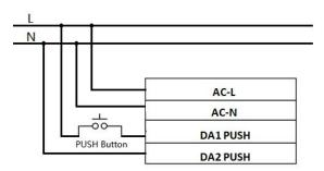
A Remark: Before using PUSH dimming function, please connect AC-L/AC-N to electricity FIRST, then connect the PUSH terminal to electricity. Otherwise the PUSH terminal will be burned.
