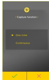
Select for one time or continuous measurement. In case continuous measurement is set, press Measurement/Local Measurement key to start auto measurement at frequency of once per 3 seconds. Press Measurement/Local Measurement key again to stop continuous measurement. (See Section 4.2: Continuous measurement for reference.)
