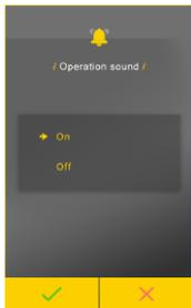
Select to on/off operation sound. Set operation sound on to beep once after measurement operation (enabled by pressing the Measurement / Local Measurement key) completed.
