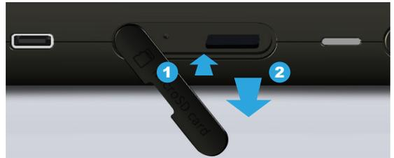
1. The SD card features a card latch design to prevent it from coming loose. You may feel that the SD card is stuck when it is inserted in or removed. In this case, pull or push it a little harder to get it in place or removed. To remove SD card: Press it as shown in step ① and pull it out after ejecting as shown in step ②.
