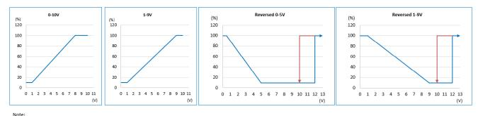
During reversed dimming mode, when the DIM+/DIM- is open, the driver will be at maximum output current.
